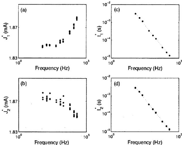
Fig. 4. Log-linear plot of the PS point for (a) increasing and (b) decreasing bias current versus the frequency of the ramp. Log-log plot of PS time for (c) increasing and (d) decreasing bias current versus the frequency of the ramp. The dashed lines indicate the linear fit  $\log(t_{1,2}^*) = a \log(f) + b$ .
