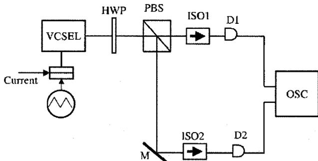
Fig. 1. Schematic diagram of experimental arrangement. HWP, half-wave plate; PBS, polarization beam splitter; ISO1, ISO2, optical isolators; D1, D2, photodetectors; M, mirror; OSC, oscilloscope.
