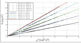
Fig. 3. Centripetal acceleration as a function of the angular velocity squared for different distances.
