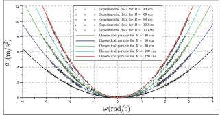
Fig. 2. Centripetal acceleration as a function of the angular velocity for different distances indicated in the legend box.
