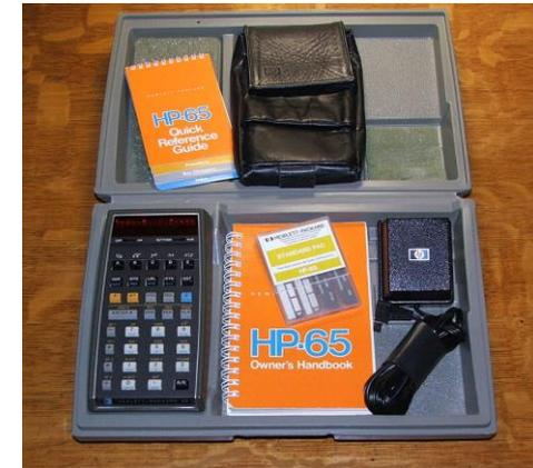
HP-65 calculator: the first magnetic card-programmable handheld calculator
