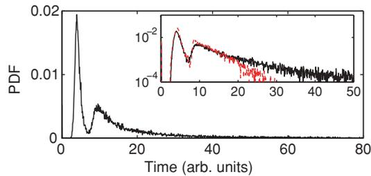
FIG. 7. (Color online) Probability distribution function for the transient time for the EMG model. Parameters are as in Fig. 6. Inset: the same plot with vertical logarithmic scale with noise (solid line) and without noise (red dashed line).
