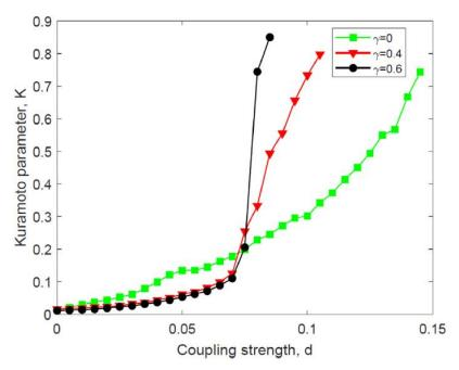
50 Kuramoto oscillators: Even when the synch transition is explosive, the lags between linked oscillators decrease faster and provide an "early warning" of the transition.
