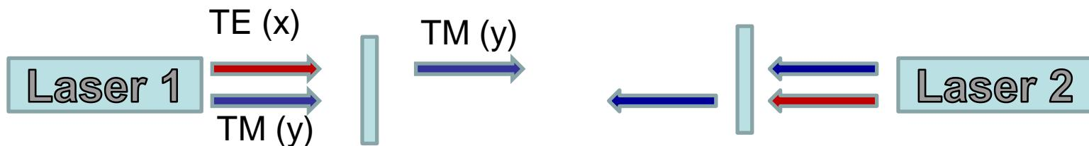
TE (x) is the natural lasing polarization of the solitary lasers.
