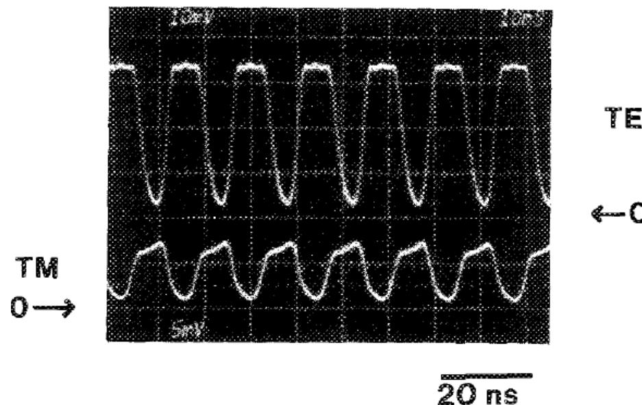
FIG. 3. Oscilloscope trace of optical pulses: upper trace: TE component, lower trace: TM component. The external cavity length is 100 cm and the current bias is 27 mA.
