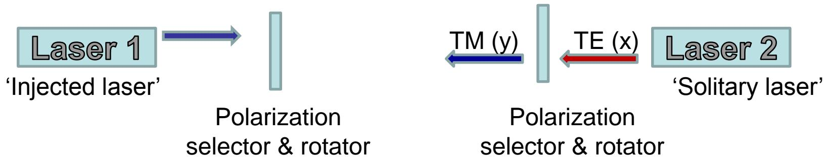
Stationary state: master-slave unidirectional coupling, Laser 2 → Laser 1
