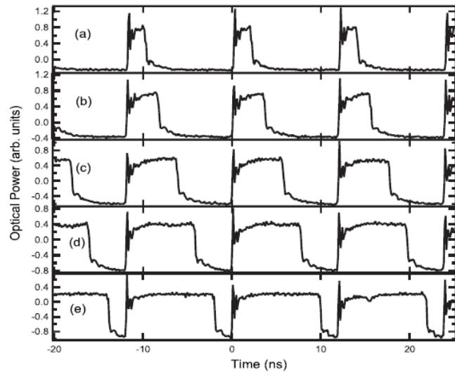
FIG. 4. Experimental square waves with variable duty cycle as a function of pump current. Only the TE mode of LD2 is illustrated for clarity.
