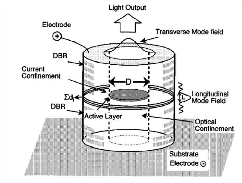
because of different cavity geometries: EELs & VCSELs have different polarization properties
