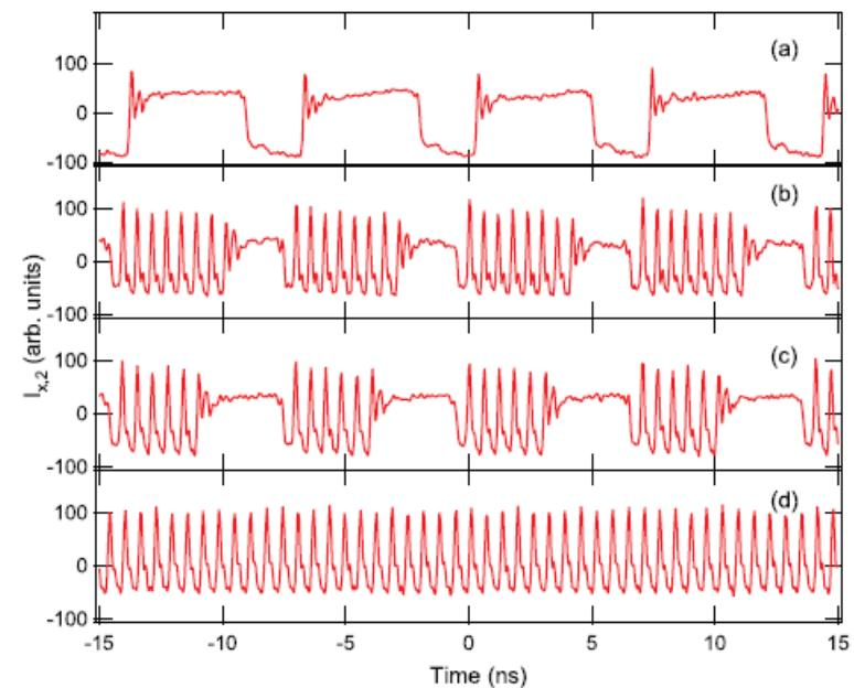
Time traces of the intensity of one mode of one laser
