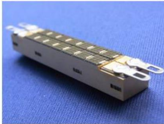
Submodule with 12 x 14 chips on sub-mounts on a micro-channel cooler
