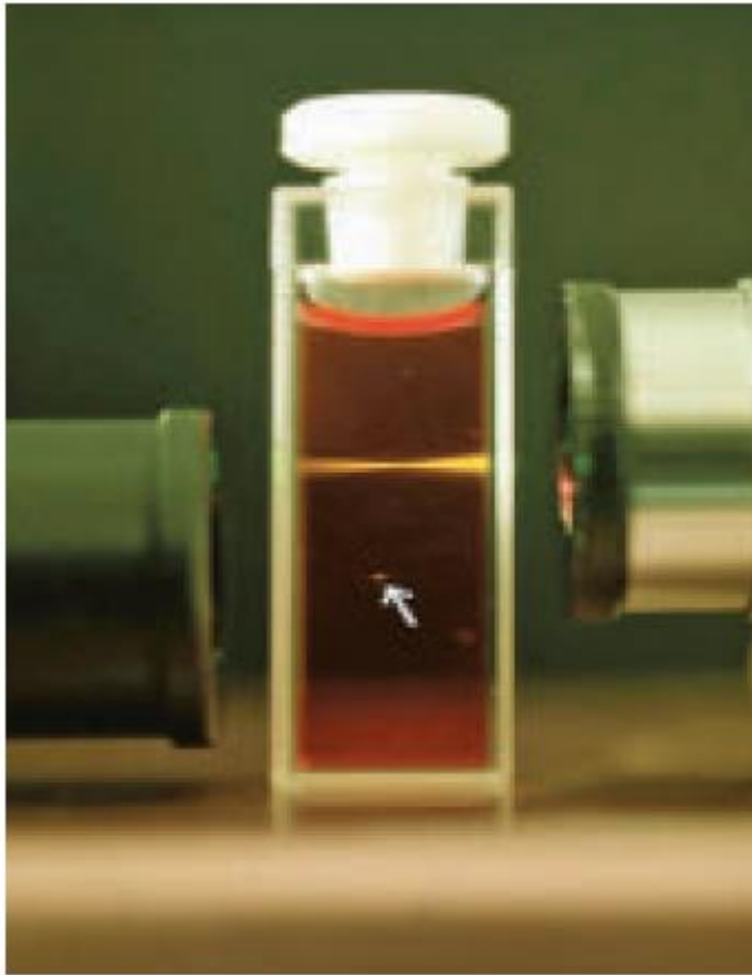
FIGURE 1. Nonlinear microscopy has inherent 3D capabilities. With a green beam (532 nm) coming from the right, single-photon absorption excites fluorescence along the entire light path. But with a near-infrared (NIR) beam (1057 nm) coming from the left, two-photon absorption excites fluorescence only at the small intense focal spot indicated by the arrow. (Image courtesy of Brad Amos, Science Photo Library, London)
