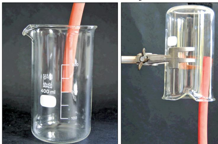
Fig. 1. In physics labs with different gases (left: heavier than air; right: lighter than air).
