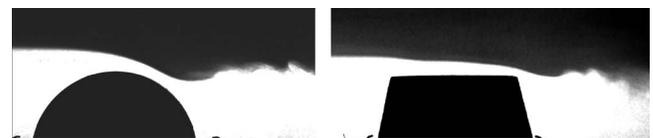
FIG. 9. Flow passing over the two obstacles of different geometry. These snapshots correspond to the KH instability between both layers at  $F_0 = 0.102$  for the prismatic obstacle and at  $F_0 = 0.064$  for the semicylindrical obstacle.
