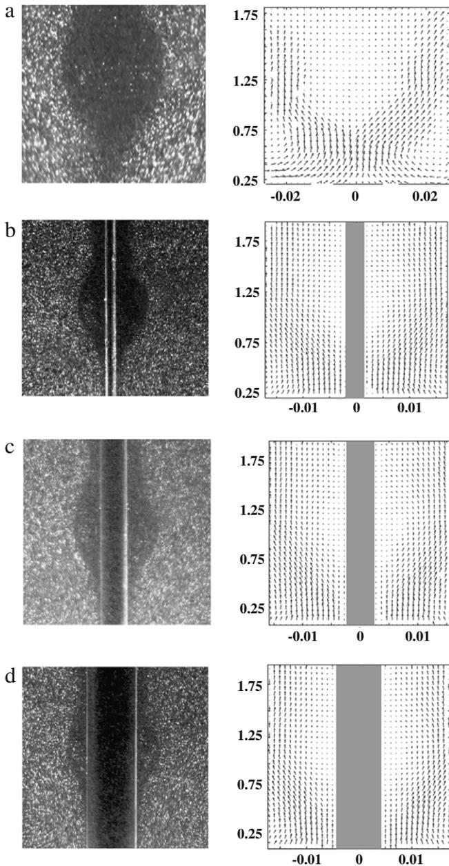
**Fig. 2.** PIV images and velocity fields of the region in which the recirculation bubble is located at the onset of VB for different radius of the rod. The aspect ratio ( $H/R = 2$ ) is the same in all the images while the  $Re_c$  varies in each image: (a)  $Re = 1474$ , without rod; (b)  $Re = 1313$ ,  $R_r/R = 0.025$ ; (c)  $Re = 1431$ ,  $R_r/R = 0.0625$ ; (d)  $Re = 1671$ ,  $R_r/R = 0.125$ .
