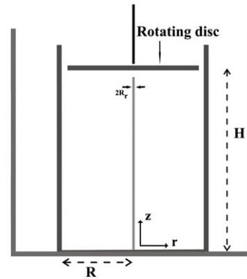
Fig. 1. The experimental setup consists of a closed cylinder, radius  $R$  and height  $H$ , with a rotating top wall. Along the axis of the cylinder a stationary rod of radius  $R_r$  is located. An external container was used in order to minimize the optical distortion of the images due to the curvature of the cylindrical wall.
