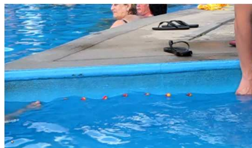
Figure 5. Wave-profile measuring device made of a set of equally spaced floats joined by fishing line. Here, the device was placed near the edge of the pool to keep the floats in line. Still photographs enabled the identification of wave profiles and wavelengths, while video recording was used to determine periods.
