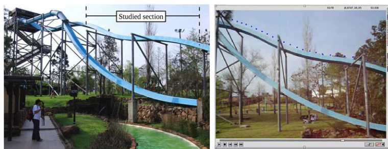
Figure 1. Overview of the Acuamanía park water slides (left) and screen shot of the LoggerPro software showing the position of the participant at different times (right). The section of the water slide analysed by the LoggerPro is schematically indicated in the left panel. The green vertical line in the background of the right panel, under the chute, was used as a reference scale, in this case the height of a sunshade pole.
