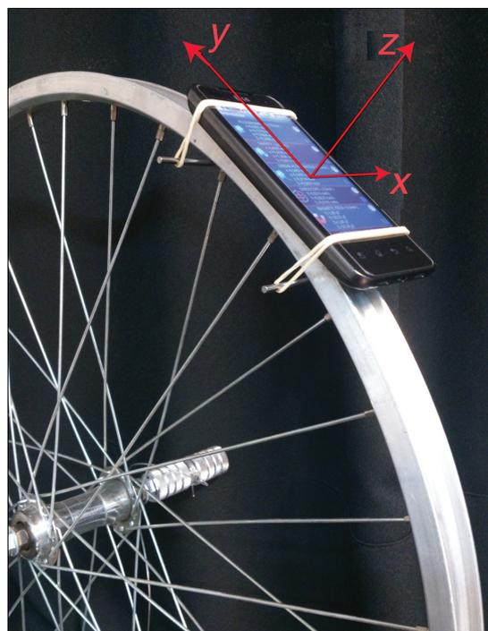
Fig. 1. Smartphone mounted on a bike wheel and a scheme indicating the axes orientation.
