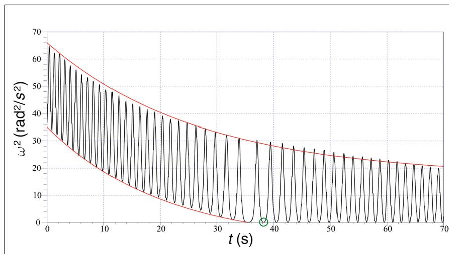
**Fig. 2.** Angular velocity squared (black), proportional to the kinetic energy, and two exponential curves fitting relative maxima and minima (red). The green circle indicates the transition from rotations to oscillations.
