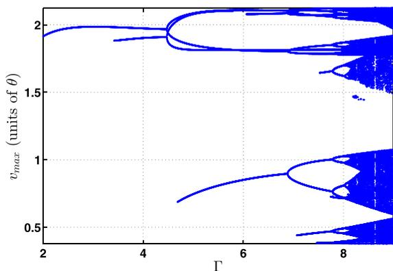
FIG. 6. Bifurcation diagram displaying the maxima of time series, as a function of the normalized delay,  $\Gamma = \tau/RC = Ndt/RC$ , obtained from simulations of Eq. (6).  $\alpha = 3.73$ , other parameters are as in Fig. 3.
