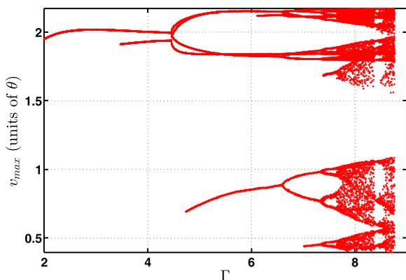
FIG. 7. Empirical bifurcation diagram. The electronic circuit delay line has  $N = 1194 C = 1.0 \mu\text{F}$  capacitors. To vary  $\Gamma = \tau/RC = Ndt/RC$  within the same range as Fig. 6,  $R$  was varied in the range  $0.5 \text{ k}\Omega - 1.0 \text{ k}\Omega$  and  $\alpha = 3.73$ , as in Fig. 6.
