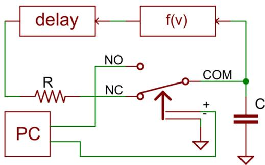
FIG. 1. Experimental setup. The electronic circuit consists of two passive elements,  $R$  and  $C$ , and two blocks, one implements the nonlinear function,  $f(v)$ , and the other the delay. The initial conditions can be arbitrarily set by using the relay which allows to switch between a free evolution in the NC position, and a controlled evolution in the NO position. The relay state and the voltage in the NC position are controlled by a PC.
