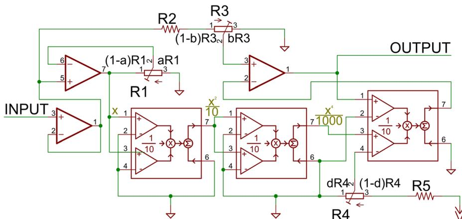
FIG. 2. Electronic implementation of the nonlinear function. Resistor values:  $R_1 = 20 \text{ k}\Omega$ ,  $R_2 = 56 \text{ k}\Omega$ ,  $R_3 = 20 \text{ k}\Omega$ ,  $R_4 = 2 \text{ k}\Omega$ , and  $R_5 = 56 \text{ k}\Omega$ .
