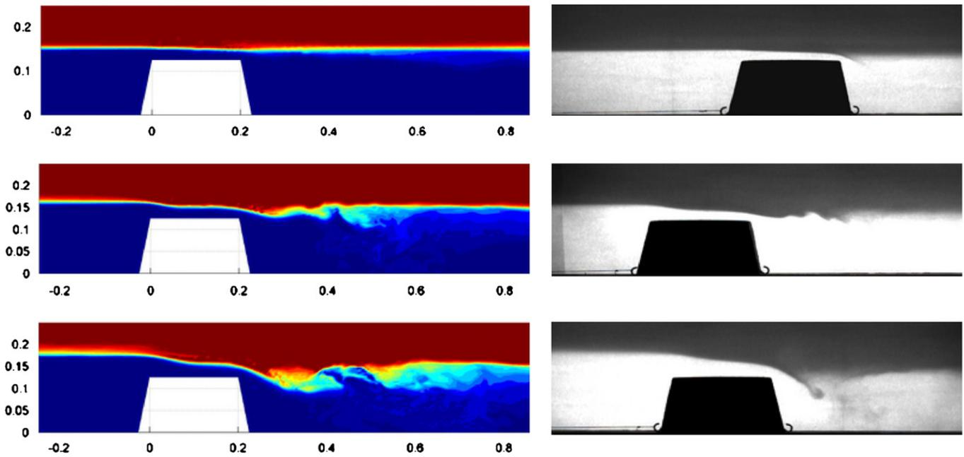
Fig. 2. Numerical simulations of a flow, from left to right, past an obstacle (left) and experiments of a leftward moving obstacle (right) corresponding to  $d_1 = 0.10$  m (upper layer),  $d_2 = 0.15$  m (bottom layer) and three different velocities: (a)  $U = 0.16$  cm/s (top), (b)  $U = 0.38$  cm/s (middle) and (c)  $U = 0.64$  cm/s (bottom).
