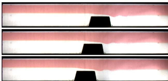
Fig. 1. Flow over the leftward moving obstacle for  $d_2 = 15 \text{ cm}$  (bottom layer),  $d_1 = 10 \text{ cm}$  (top layer) and  $U = 0.30 \text{ cm/s}$ . Three different snapshots covering the whole channel are shown.
