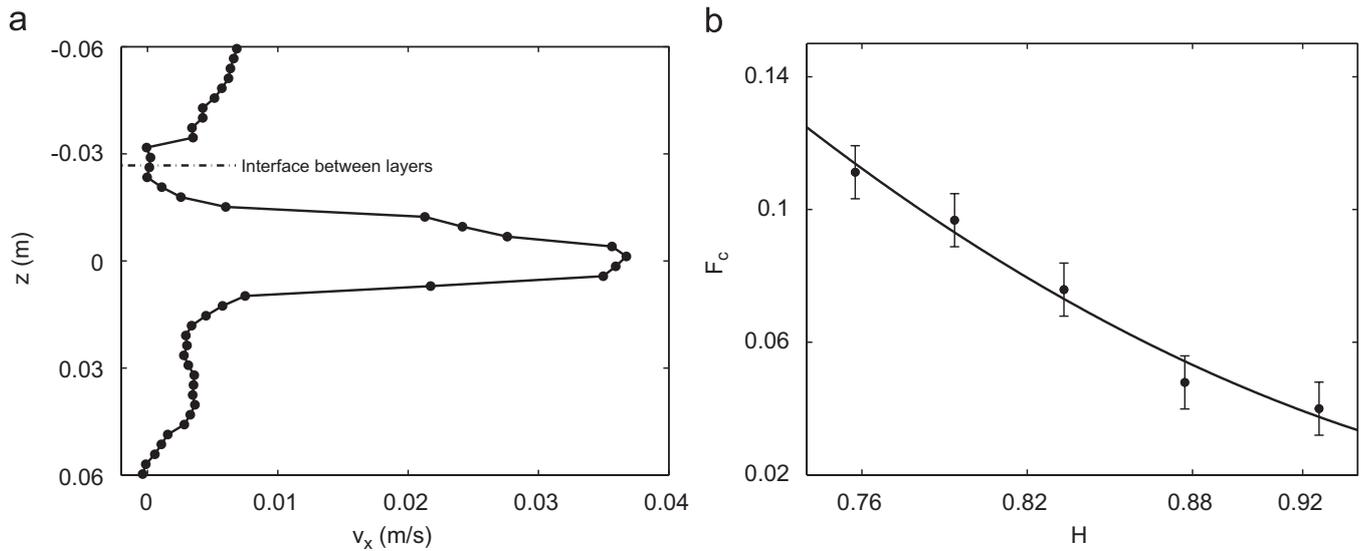
Fig. 3. (a) Experimental profile of the horizontal velocity near the interface at the end of the obstacle as a function of the vertical coordinate  $z$  obtained from PIV for  $F_0 = 0.076$  and  $H = \frac{5}{6}$ . (b) Critical Froude number for the emergence of shear instability as a function of  $H$ . The points and error bars correspond to the experimental values.
