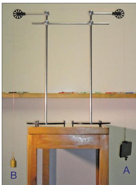
Fig. 1. Experimental setup consisting of two supports (A) and (B), connected by a string and supported on two pulleys.
