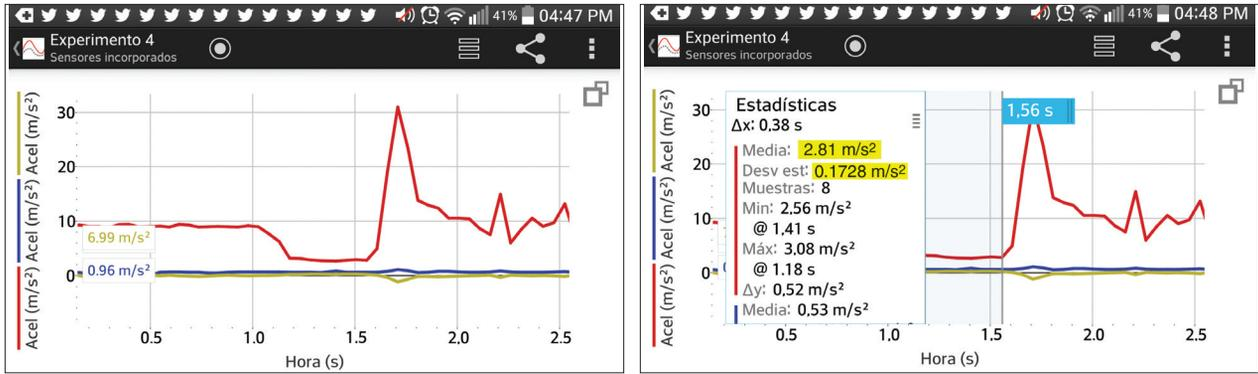
Fig. 4. Snapshots of the Vernier app showing the values registered by the acceleration sensor as a function of time. The only relevant component here is the  $x$ , which corresponds to the vertical acceleration. On the left panel, the plateau of constant acceleration can be appreciated. The statistical values (mean and standard deviation) calculated for this interval are highlighted in the right panel above.
