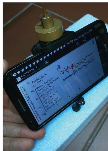
Fig. 3. Smartphone mounted on the support showing the Vernier app on the screen.
