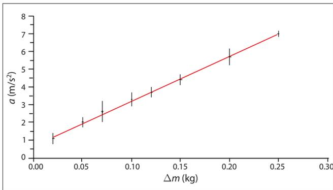
Fig. 5. Acceleration as a function of the mass difference: experimental points with error bars (black) and a linear regression (red line). Note that the yellow highlighted results from Fig. 4 are included here as the right-most data point after subtracting the acceleration due to gravity ( $9.8 \text{ m/s}^2 - 2.81 \text{ m/s}^2 \approx 7.0 \text{ m/s}^2$ ).
