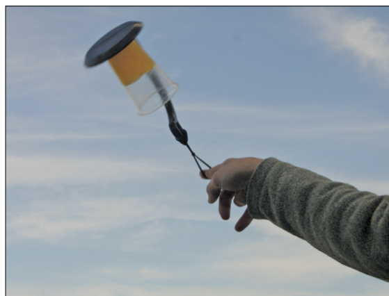
Fig. 1. Snapshot showing a cup on a SpillNot giving full turns in a vertical plane; the surface of the liquid can be appreciated.
