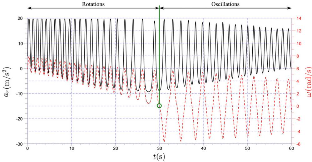
**Figure 2.** Radial acceleration (left axis, black lines) and angular velocity (right axis, red lines). At the initial stage when there is enough energy, the wheel is rotating. At the point indicated with the green circle, the angular velocity changes its sign and the wheel starts oscillating about the stable equilibrium point.
