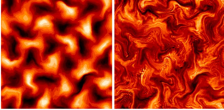
Fig. 1. Scalar concentration, for  $s = 0.34$  and  $\alpha = 0.25$  (left) and  $\alpha = 0.025$  (right). The parameter of the velocity field are  $u_0^2 = 4.0$ ,  $t_0 = 5.6$ , and  $l_0 = 8.0$ ,  $N = 256$ , and  $\Delta = 0.5$ .
