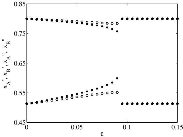
Fig. 2. Dependence of  $x'_A, x'_B$  (circles),  $x''_A, x''_B$  (stars) with the coupling strength. We chose the *same* random initial condition for all  $\epsilon$ . Above a certain threshold,  $\epsilon \approx 0.09$ , the data stand for the states of the in-phase solution. The parameters are  $N = 100$ ,  $a = 3.2$ , and  $k = 2$ .
